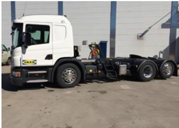
IKEA's road tractor and the flexi-trucks are produced by Scania and equipped with fully automatic Allison 3000 Series™ transmissions. The trucks also feature a moved forward, low-entry cab.
