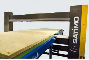
immediately detecting defects in any sort of non-metallic material.
