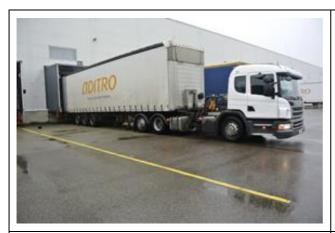
The difference between road tractors and flexitrucks is that the flexi-trucks also can carry swap bodies. Both are equipped with Allison transmissions.
