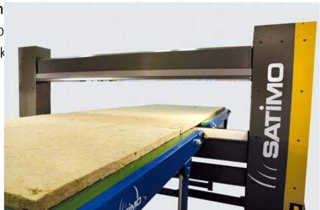
Microwave imagery, in combination with computerized data processing, enables this process to take place in real time. This technology is completely safe for the environment, and eliminates any health risk to operators, as opposed to scanners using X-rays or gamma rays.
